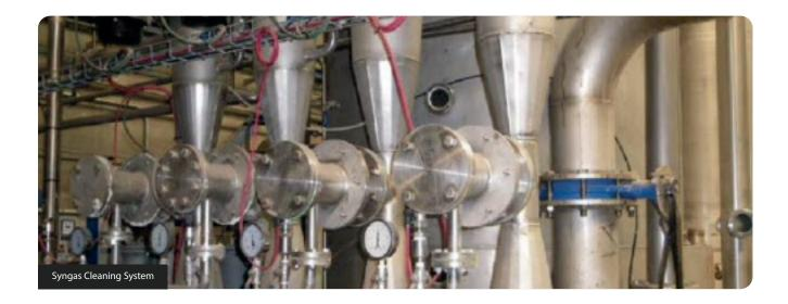
Among the several conditioning steps, our thermal cracking and reforming reactor is key. It creates the conditions necessary to maximize the production of H2 and CO, which ensures the high quality of the syngas. The reactor also reduces the tars in the syngas stream, avoiding problems in the downstream equipment while also recovering part of the energy of these compounds.
